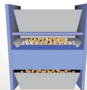
Material released from the gated Universal Splitter Hopper flows evenly across the entire width of the chutes.
