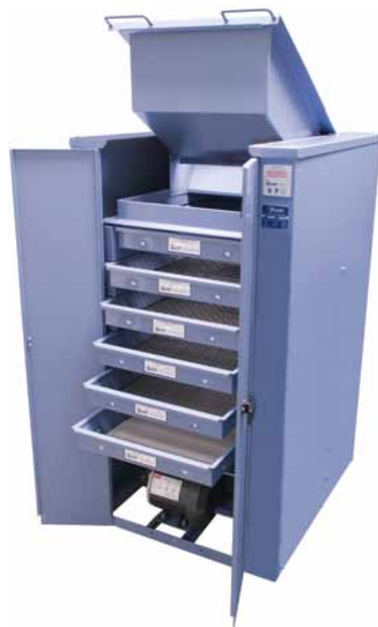
TM-5 shown with Screen Trays. Doors open & Hopper elevated
