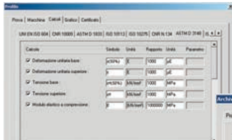
A150N Selection of the test Standard with possibility to personalize the calculation algorithm
