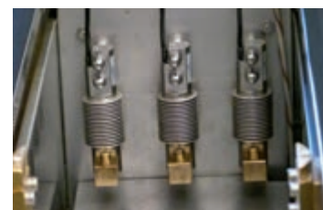
Detail: 3 load cells 500 N
