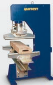
FLEXURAL TEST WITH THE OPEN SIDE FRAME
